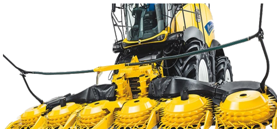
New Holland FR920 Corn chopper FPT Vector20: 4095 Nm, 670 kW
